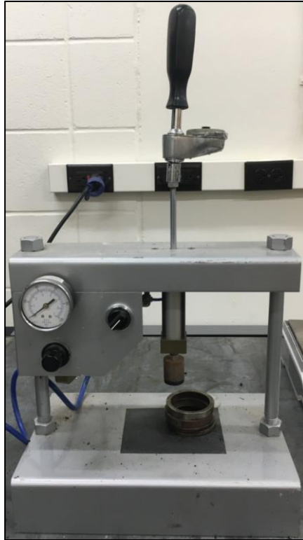
Figure 6. Cohesion Tester at Iowa State University
